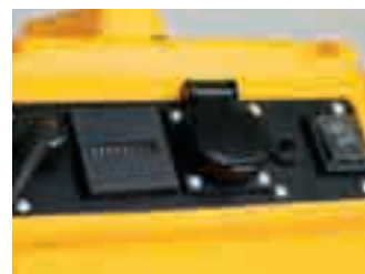
DFX 20 control panel – hour counter, extra power socket, 2 speed switch.
